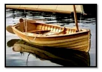
eight ten-foot 'Puffin' clinker sailing dinghies, (known for their overlapping plank or lapstrake construction). They were stacked two high; the lower boat was on chocks and rollers and slid under the top one. He had me operate the air-hoist while pushing the boat out over the water. The boat owner would usually go down the ladder to get in and install the mast and rudder. He told
